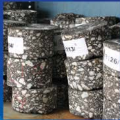
Asphalt Premix Testing
